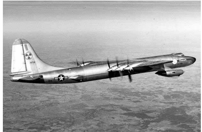
A modified B-36 Bomber became the United States’ only flying nuclear reactor in 1955. It carried a small air-cooled reactor in the aft bomb bay.
