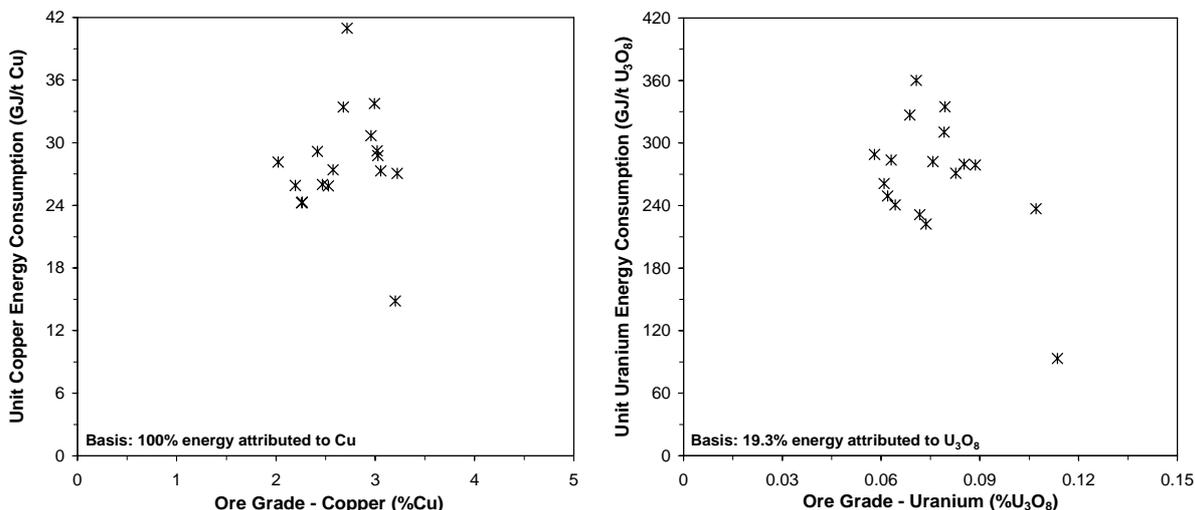
Figure 7: Unit energy consumption versus ore grades – copper (left) and uranium (right)
