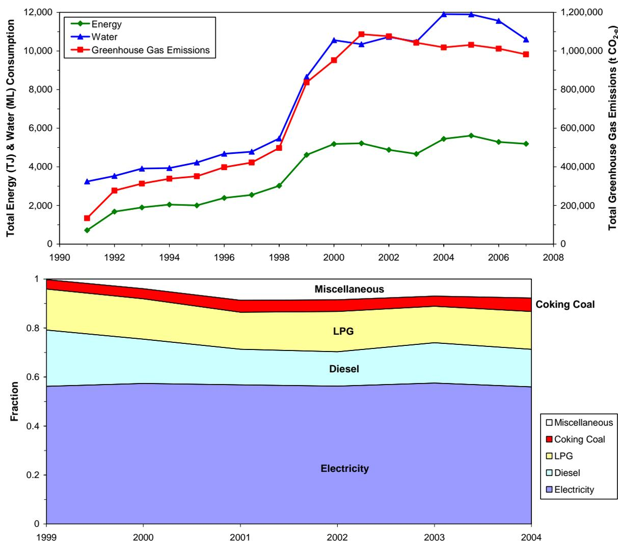
Figure 5: Annual energy consumption and greenhouse gas emissions for Olympic Dam (top) and energy source by fraction (1999-2004; bottom) (1991 to 2007; with years 1998 to 2004 being calendar year, all others are financial year)
