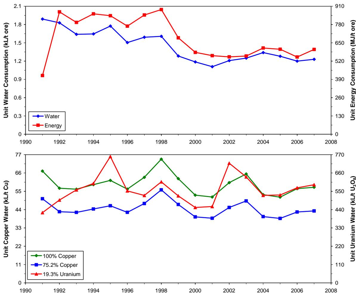
Figure 8: Water and energy costs in processing ore at Olympic Dam
