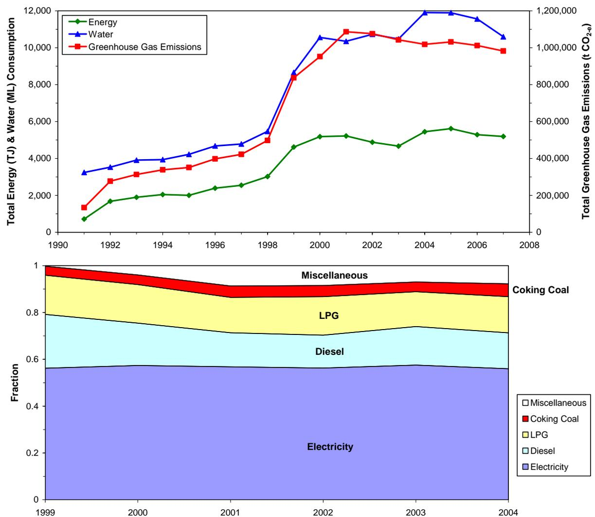
Figure 5: Annual energy consumption and greenhouse gas emissions for Olympic Dam (top) and energy source by fraction (1999-2004; bottom)
