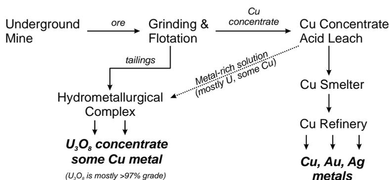
Figure 1: Conceptual representation of the process for treating ore at Olympic Dam (adapted from Kinhill, 1997)
